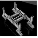
The VariWidth system features rollers and hydraulic clamping pucks to easily extend and retract tractor extension tubes without supports. VariWidth can cut tractor width change time from hours to minutes.
