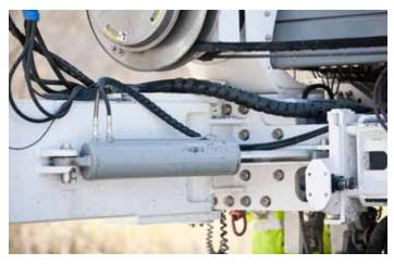
The SmartLeg system allows contractors to adjust the swing leg angle on-the-fly to maneuver around an obstacle without stopping production.
