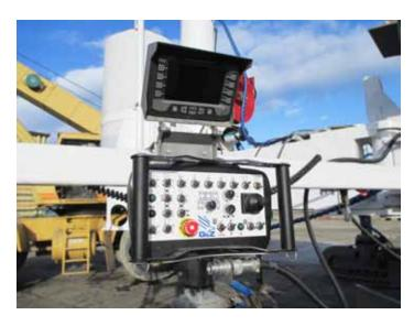
EGON Belly Pack console provides great flexibility to the operator. With the option to mount the entire console with the LCD display on any sensor arm or take the console remote, the EGON Belly
